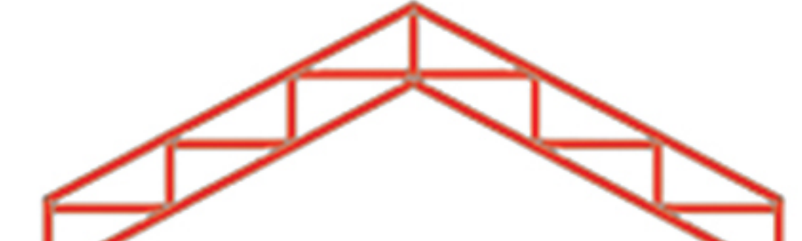
Parallel Chord Truss
