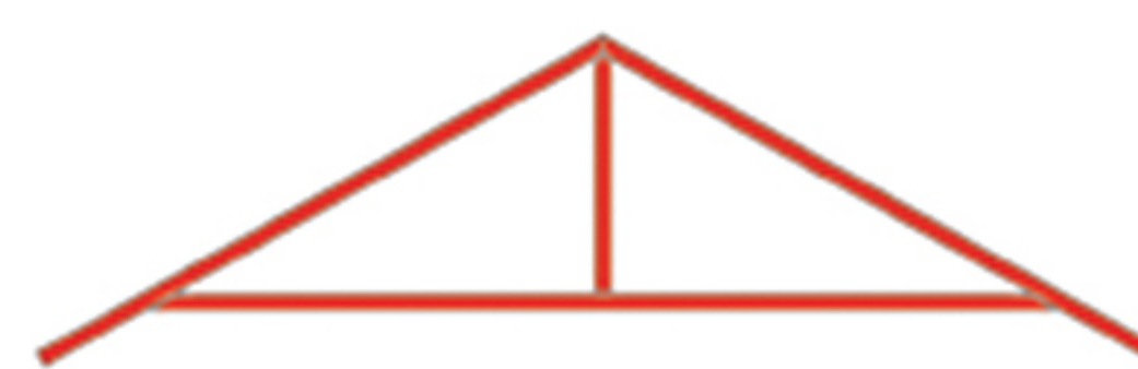
King Post Truss
